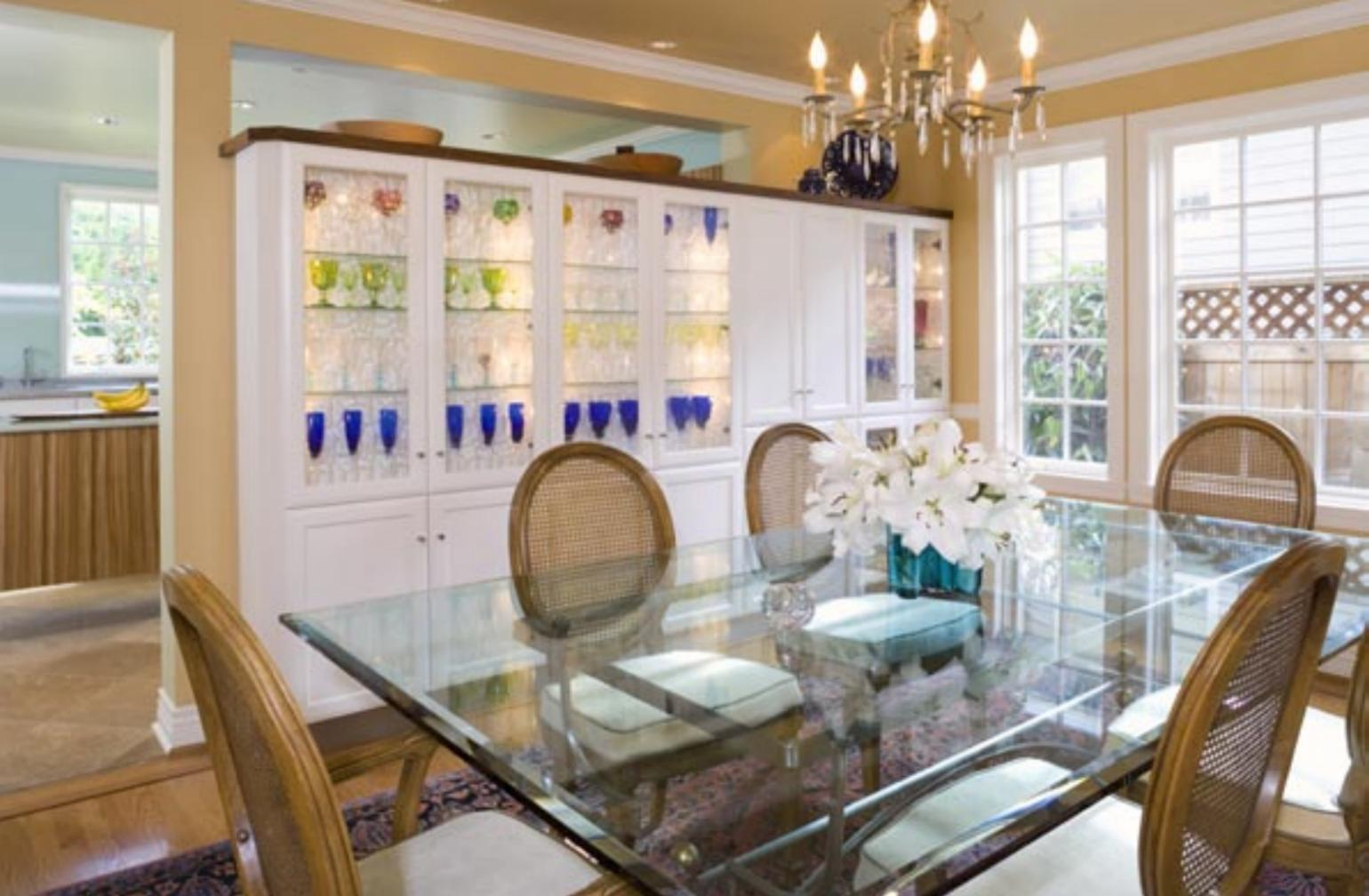
**TOP LEFT & RIGHT** Removing the wall between the dining room and kitchen opened up the Light and View Pathways. Note the many ways that glass affects the composition. Moving the window headers up into the second-floor rim joists made these windows 8" taller, filling the room with daylight! The chef's sink also serves an adjacent prep counter.
